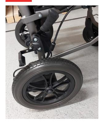
When parking on a ramp, the electromagnetic brake may not always be strong enough. Always use the manual brake in conjunction with the electromagnetic brake.
