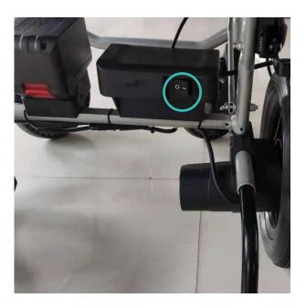
Switch off the main power supply from the control box at the back of the power chair.
